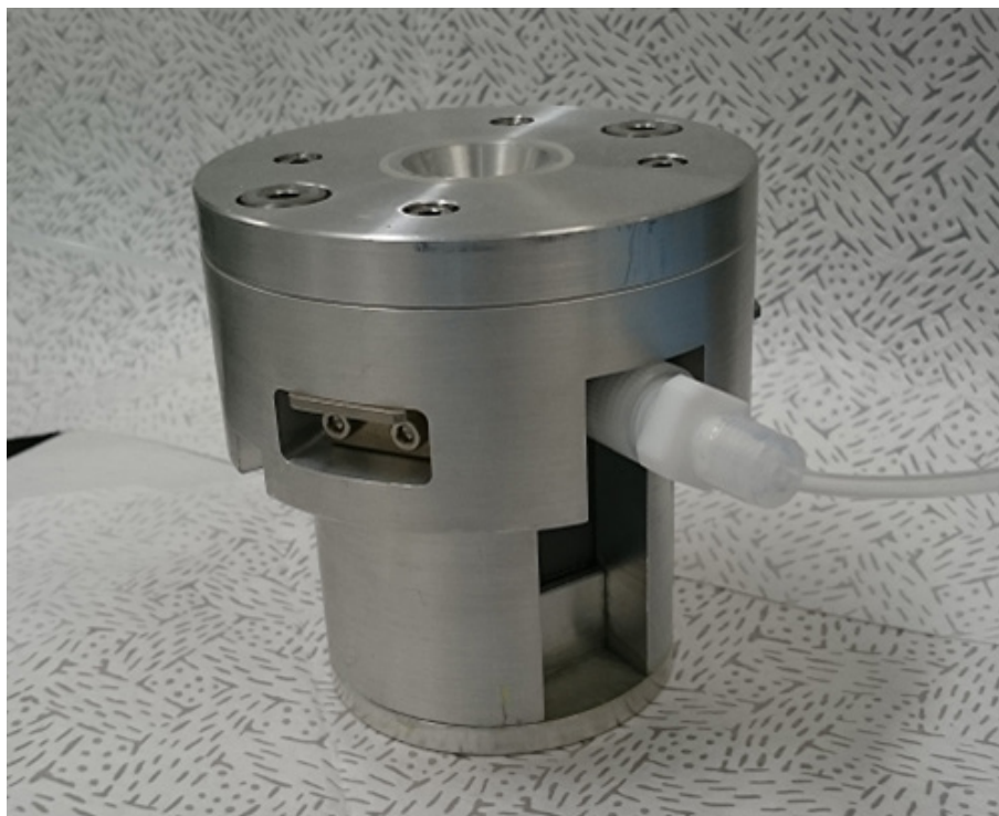
FIG. 21. Developed target vessel made of SiC and its holder for a vertical irradiation system.
